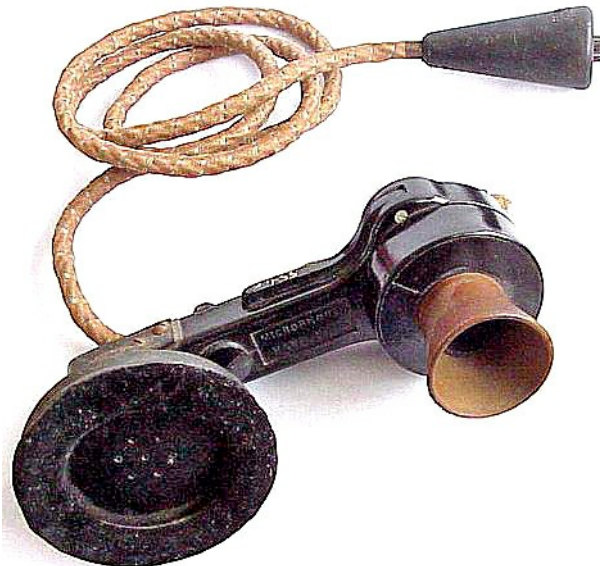
Mechanical arrangements of fitting a single earpiece to the dynamic type Microphone Hand No. 7. Both were originally part of Microphone and Headgear Assembly No. 1.
