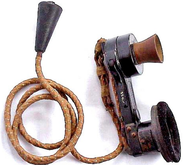
Mechanical arrangements of fitting a single earpiece to the dynamic type Microphone Hand No. 7. Both were originally part of Microphone and Headgear Assembly No. 1.
