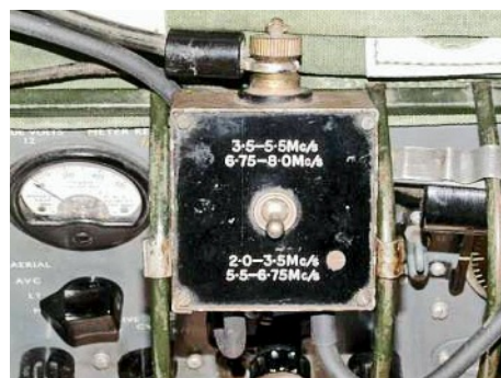
Photograph of Aerial Coupling Unit No. 4, clamped on the Wireless Set No. 22 grille. Three versions of this unit were noted: Mk.I (ZA 10560), Mk.II (ZA 22594) and Mk.IIT (ZA 27322), differing only in small detail.
