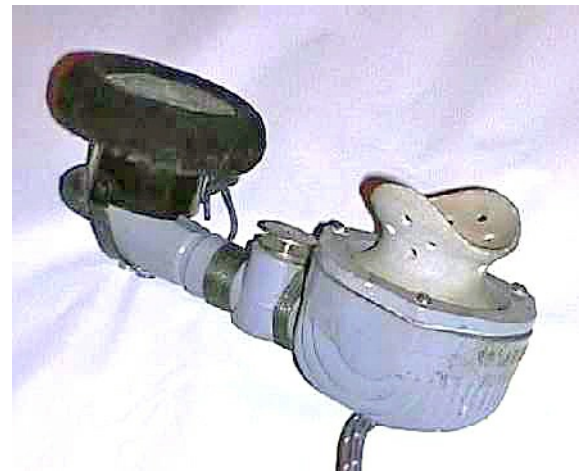
Alternative arrangements of fitting a single earpiece to a carbon granule (Tannoy) type Microphone Hand Power No. 1A, part of Microphone and Headgear Assembly No. 2. The microphone was slightly modified by two machined flat surfaces on the handle, to which was bolted the bracket for the microphone, part of the standard headset headband. The VAOS number YA 28968 was handwritten on the end of the microphone. Pictures courtesy Chris Clotworthy GI7TEU.
