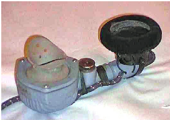
Alternative arrangements of fitting a single earpiece to a carbon granule (Tannoy) type Microphone Hand Power No. 1A, part of Microphone and Headgear Assembly No. 2. The microphone was slightly modified by two machined flat surfaces on the handle, to which was bolted the bracket for the microphone, part of the standard headset headband. The VAOS number YA 28968 was handwritten on the end of the microphone. Pictures courtesy Chris Clotworthy GI7TEU.
